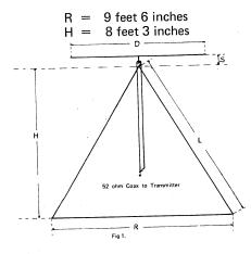
The mast section, which may be of wood or metal, is fully supported by the multiple wires forming the cone. If a metal support is used the coax could be fed through the pipe and, therefore, automatically preventing any possible feed line radiation — the balance of the coax being buried for convenience.
